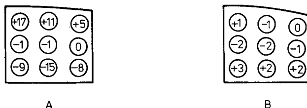
Fig. 7. Surface carrier concentration uniformity maps (using 0.1M Tiron electrolyte) for VPE n-GaAs specimens grown under different conditions. The figures represent percentage deviations from the mean values of 6.9 and 9.7 \times 10^{16} \text{ cm}^{-3} for A and B respectively.
