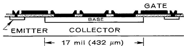
Fig. 2. Cross-sectional view of the base-collector diode used for the junction C-V measurements of dopant density.
