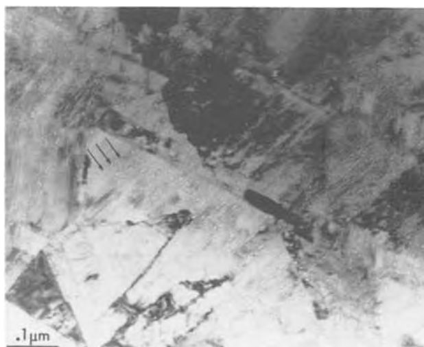
Fig. 4. Microstructure of an electrodeposited cobalt film (HP-Co) obtained in a solution with \text{pH} = 5.7 . Three arrows indicate the presence of inclusions (seen as white dot surrounded by a black ring), trapped in the (0001) basal plane of hcp cobalt grains. The micrograph is slightly underfocused to reveal the image of inclusions using the defocus contrast technique.
