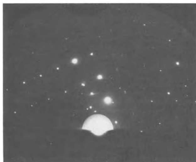
Fig. 4. SEM/RED for a 2 μm thick ZnO film grown at 400°C by the DEZ/H 2 O/H 2 growth process.
