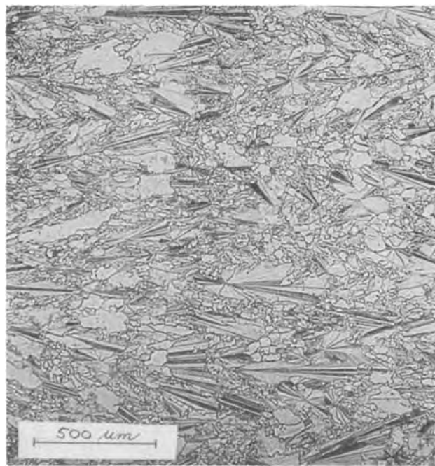
Fig. 6. Grains of material B after recrystallization at 1380^\circ\text{C} during 3 hr. The sample is sawn parallel to the original growth direction which is from left to right on the micrograph.
