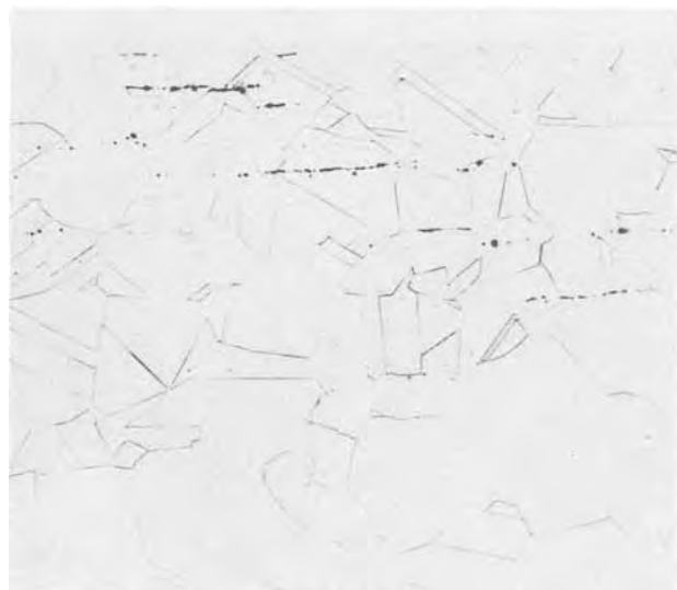
Fig. 12. Microstructure of Cu-50%Mn alloy \times 200 etched in HCl-picric acid in isopropanol.
