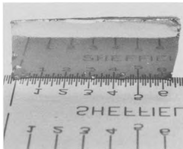
Fig. 3. The surface of an HgCdTe epilayer grown on an (111)Cd oriented substrate. The number scale is 0.1 in.
