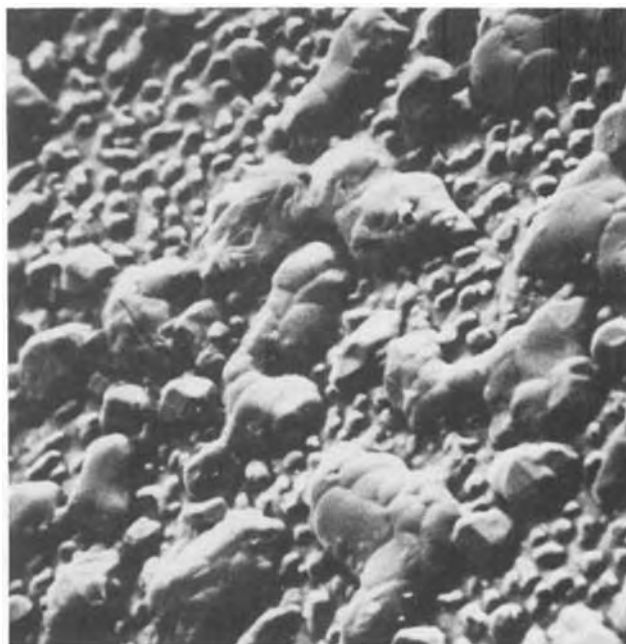
Fig. 18. A demixed cathode, after long term operation under 50% H 2 O + 50% H 2 at 900°C.
