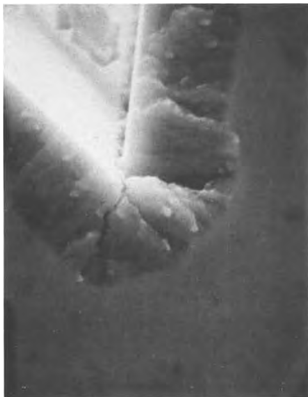
Fig. 8b and c. Enlargements of two regions at the intersection of two CdS planes (5000 \times )
