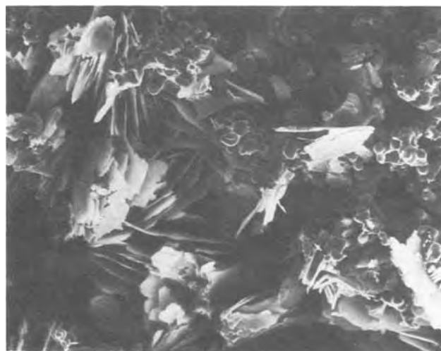
Fig. 12. Scanning electron micrograph of nickel plaque impregnated with \text{Cd}(\text{OH})_2 . Low current densities ( 0.2\text{ A/in.}^2 ) employed in this deposition never allowed the electrode to become more negative than -0.65\text{V vs. SCE} . \text{Cd}(\text{OH})_2 platelets are seen to be imbedded within the pores of the sintered nickel plaque material.
