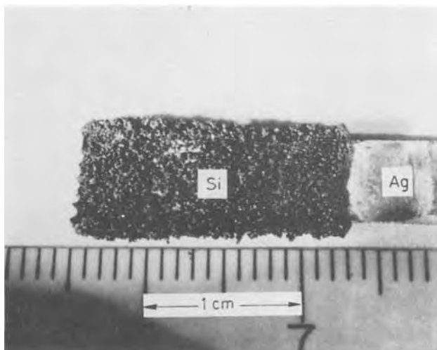
Fig. 5. General view of thick deposit plated at constant cell potential of -1.9\text{V} vs. Pt at 750^\circ\text{C} , the \text{K}_2\text{SiF}_6 concentration \sim 2.5 m/o.
