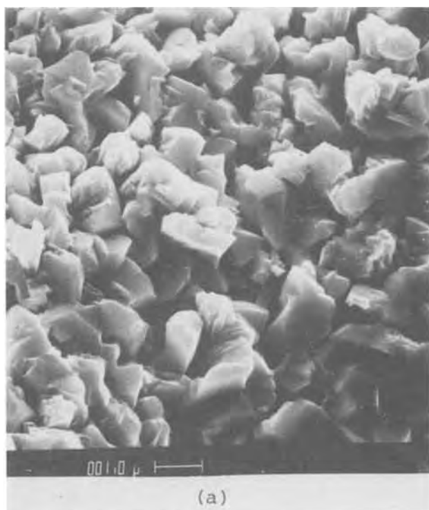
Fig. 5. Scanning electron micrographs of \text{Bi}_2\text{Ru}_2\text{O}_7 electrode (a) before \text{Cl}_2 evolution and (b) after \text{Cl}_2 evolution. Scale is 1 \mu\text{m}
