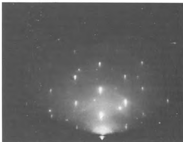
Fig. 6. SEM/RED for a 1.5 \mu\text{m} thick ZnO film grown at 730°C by the DEZ/ \text{N}_2\text{O}/\text{N}_2 growth system.
