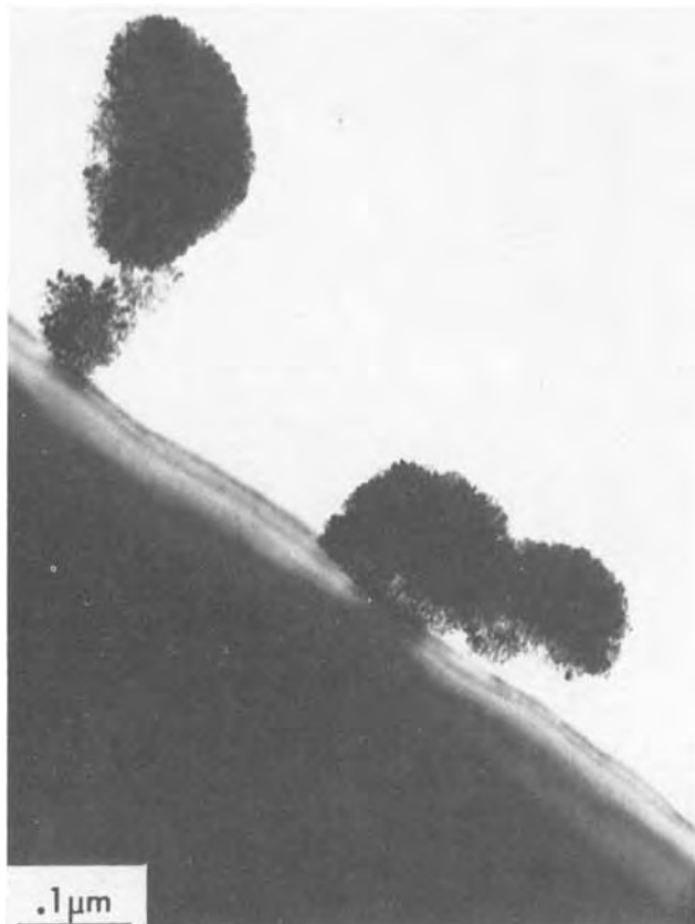
Fig. 6. TEM micrograph showing spongy Pd deposits grown at the edge of activated (111) Si foil. To reveal porous regions in the deposit, the image was taken in a slightly underfocused condition.
