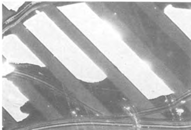
Fig. 10. A partially removed contact heated to 280°C. The dark regions are deficient in gallium. 1040 \times .
