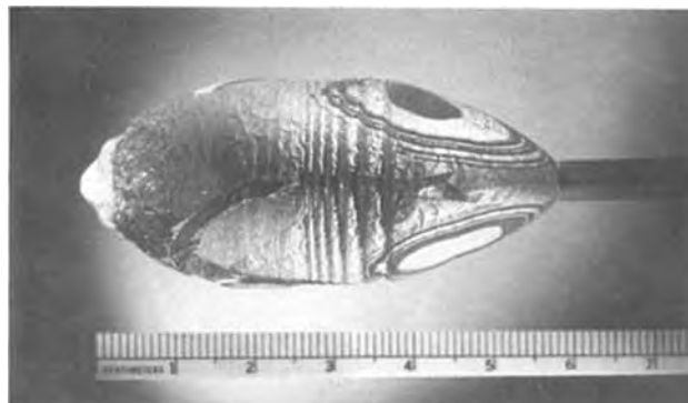
Fig. 1. InP so-called "single" crystal showing <111> parallel twin planes.
