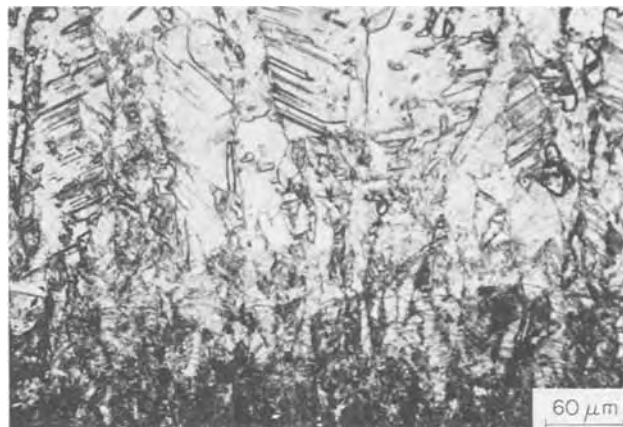
Fig. 9. Micrograph of etched silicon surface of the deposit plated at constant cathodic potential of -0.74V vs. Pt at 747^{\circ}C , the K_2SiF_6 concentration \sim 4 m/o.
