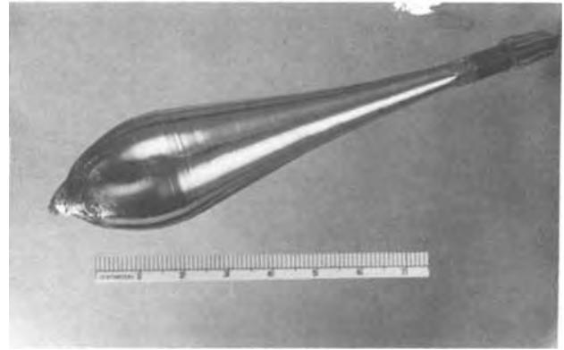
Fig. 4. Surface feature typical of twin-free InP crystal cooled at 1 atm pressure.
