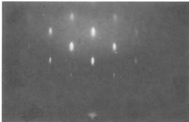
Fig. 4. RHEED pattern of ZnTe on GaAs grown at 250°C, F_1/2F_2 = 1/2 .
