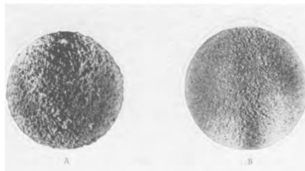
Fig. 8. Zinc deposition at and below the limiting current. 0.05M ZnCl 2 + 1.0M KCl solution.
