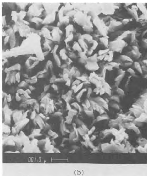
Fig. 5. Scanning electron micrographs of \text{Bi}_2\text{Ru}_2\text{O}_7 electrode (a) before \text{Cl}_2 evolution and (b) after \text{Cl}_2 evolution. Scale is 1 \mu\text{m}
