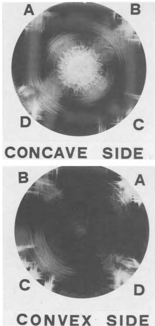
Fig. 3. Slip patterns on both sides of a plastically warped wafer delineated by Jenkins-Wright etch.
