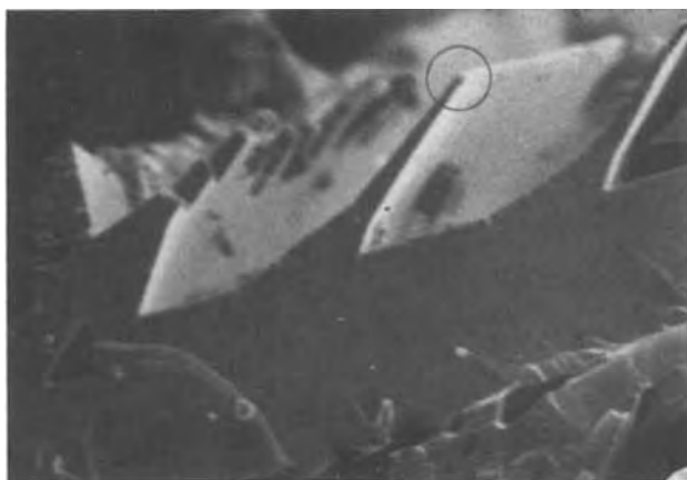
Fig. 8a. A photomicrograph of a (0001) cross section of a CdS platelet with a \text{Cu}_2\text{S} film growing on it (100 \times ).
