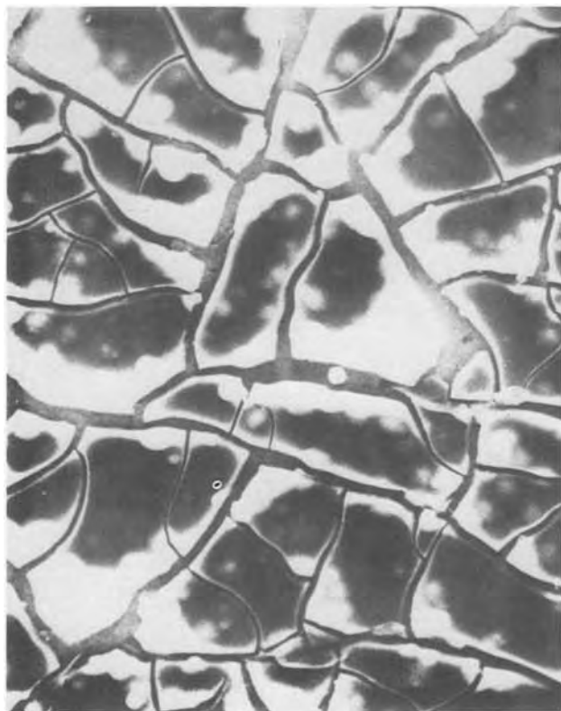
Fig. 6. SEM photograph of the cracked surface of a strongly reduced \text{Na}_{0.6}\text{WO}_3 crystal. Here the cracks can be seen to be only in the sodium depletion layer which is flaking off the crystal.
