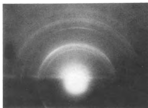
Fig. 2. Double exposure, in which Fig. 1 is superimposed onto the reference pattern of gold for measuring the interplanar spacings of the sample.
