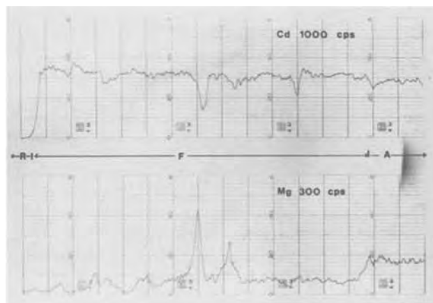
Fig. 5. Cd and Mg concentration profiles on the sample in Fig. 4. R, mounting resin; F, surface film; A, cadmium-magnesium alloy; cps, counts per second from the Electron Microprobe Analyzer.
