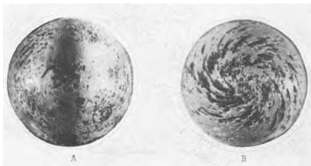
Fig. 10. Zinc deposition: the evolution of spiral markings. 0.05M ZnCl 2 + 1.0M KCl solution.
