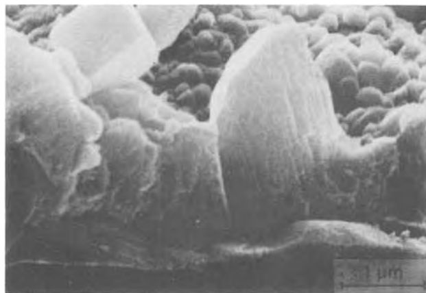
Fig. 8. Scanning electron micrograph of chromium specimen oxidized for 50 hr at 800°C and 10^5 Pa O_2 . The picture shows a fractured edge of the scale with the chromium metal beneath.
