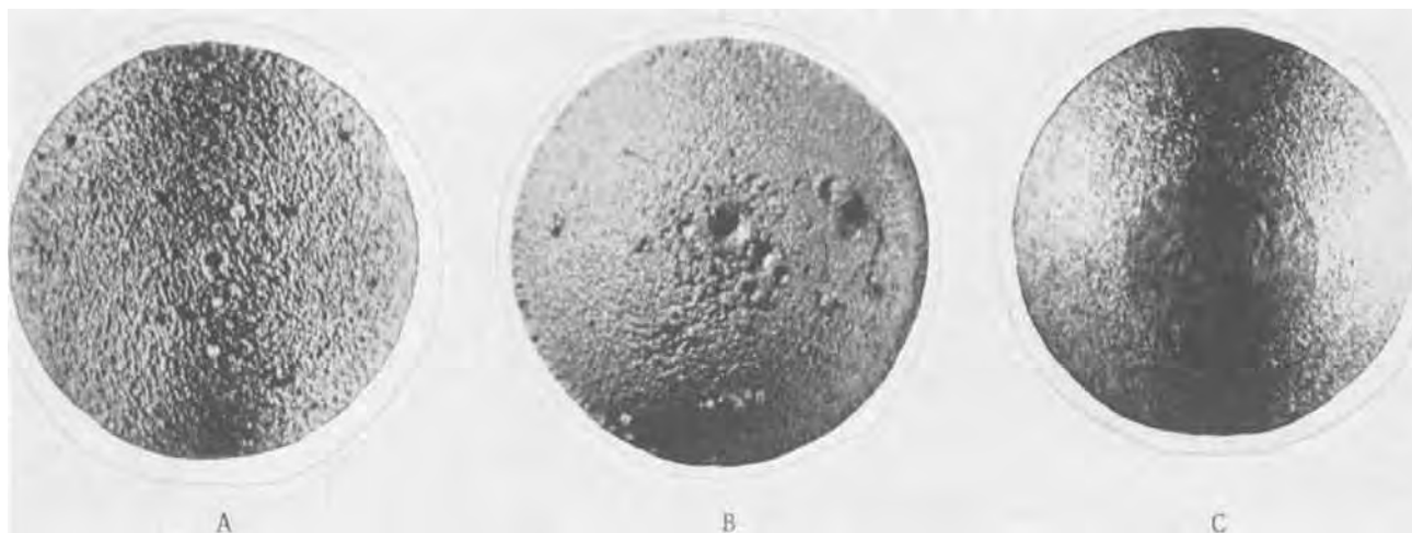
Fig. 6. Zinc deposition at different fractions of the limiting current. 0.5M ZnCl 2 + 1.0M KCl solution
