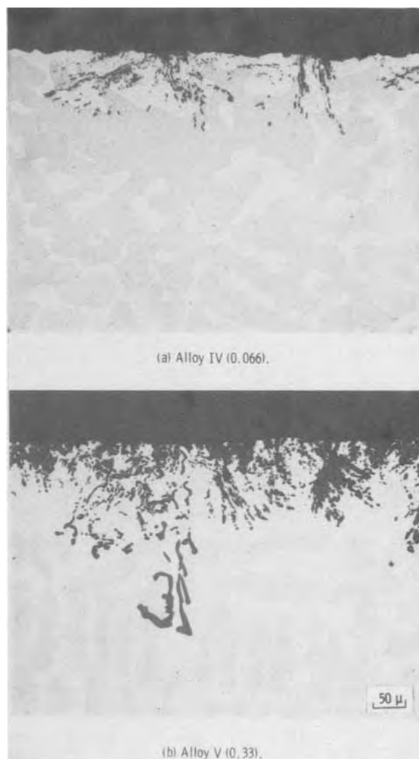
Fig. 4. Oxide penetration in Ni-14Cr-24Al-xZr. Zr contents for (a) and (b) are 0.066 and 0.33 a/o, respectively. Specimens were isothermally oxidized for 200 hr at 1150°C.
