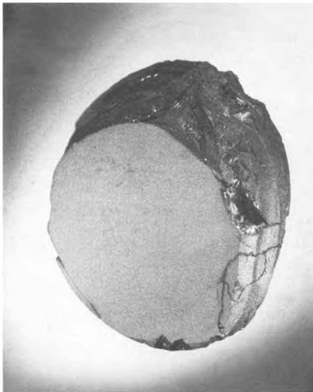
Fig. 3. \langle 111 \rangle slice through twin-free InP boule cooled at 38 atm pressure, 5\times showing extent to which surface damage can occur.
