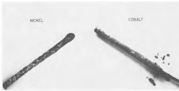
Fig. 3. Anodes from electrochemical half-cell after they had been potentiostated in Li/K carbonate melt in low BTU fuel containing 1000 ppm H 2 S at 650°C
