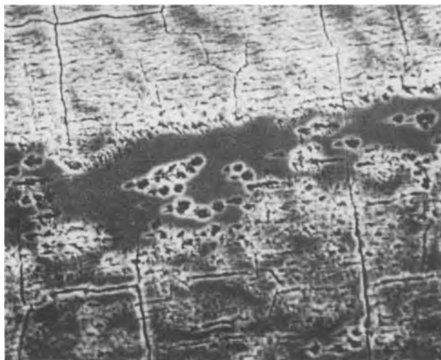
Fig. 7b. A photomicrograph of the \text{Cu}_2\text{S} film at the same intersection after being treated by a KCN etch ( 500\times ).
