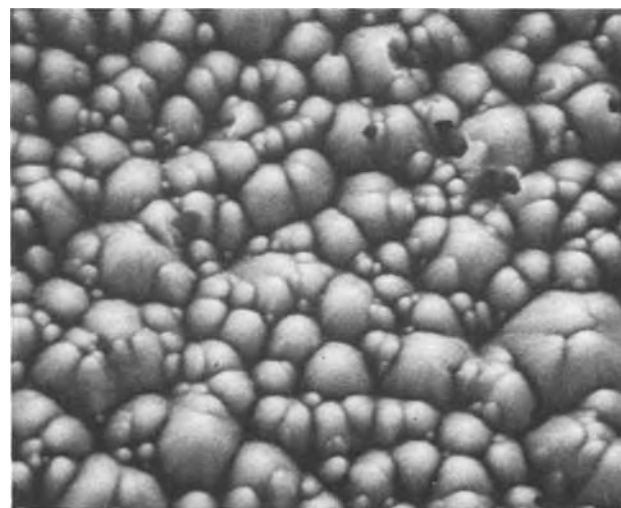
Fig. 6c. A \text{Cu}_2\text{S} film grown on an etched (0001) CdS surface ( 2000\times ).
