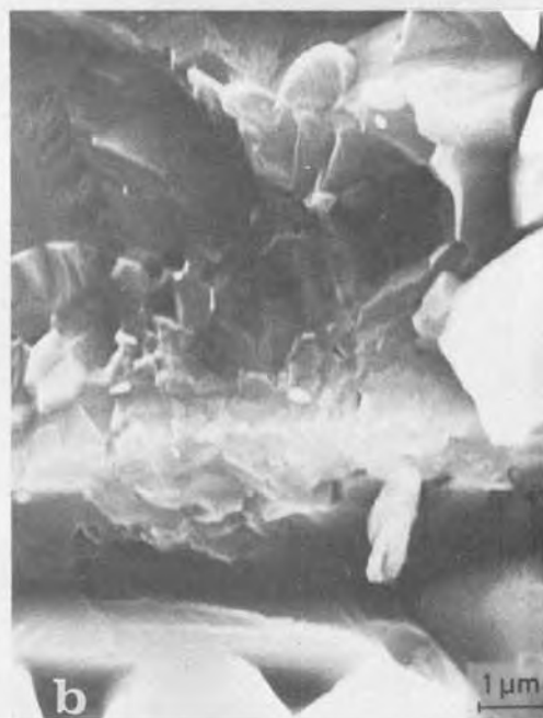
Fig. 9. Scanning electron micrograph of chromium specimen oxidized for 127 hr at 800°C and 10^5 Pa O_2 . a shows a fractured edge of the oxide scale with the metal beneath, and b a detail of a at larger magnification showing the inner surface of the scale and the surface of the metal.
