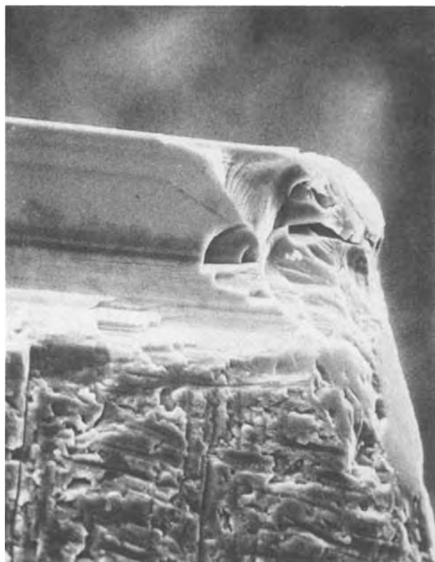
Fig. 9b. A photomicrograph of the \text{Cu}_2\text{S} film growing on the (0001) CdS plane (horizontal) and on a prismatic plane (vertical) ( 500\times ).
