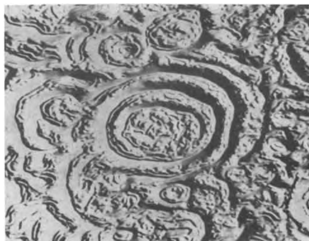
Fig. 1. A Nomarski interference contrast micrograph of a dissolved surface illustrating the two finer scale morphologies which occur. The longer side of the figure represents 680 \mu\text{m} .
