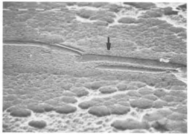
Fig. 3. This dark line structure revealed by photoetching is typical for a dark line initiated at a mirror of a GaAs-AlGaAs double heterojunction laser.
