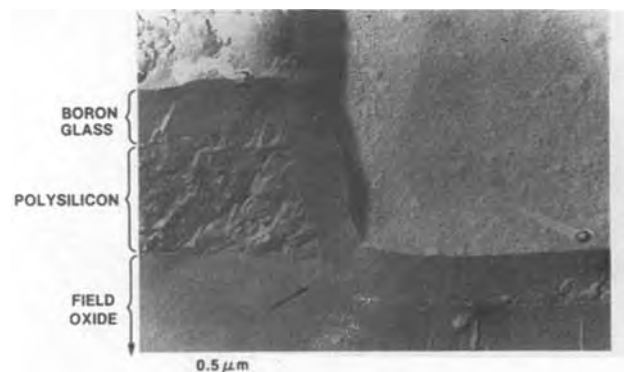
Fig. 3. TEM photo of edge fracture replica through a sample of B-glass on poly over oxide on a silicon substrate.
