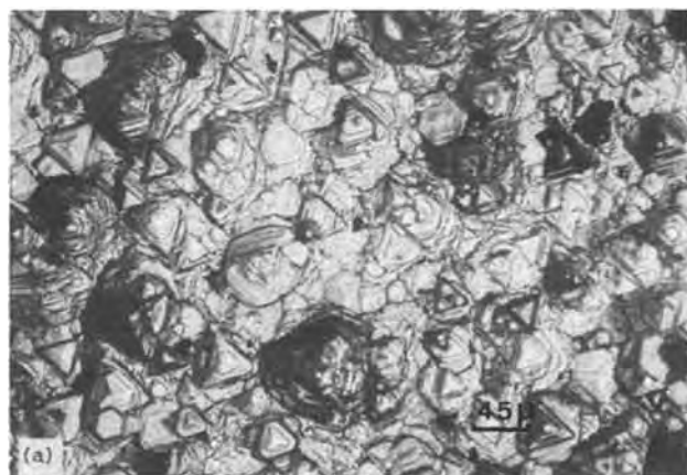
Fig. 4. Photomicrographs of \text{ZnS}_x\text{Se}_{1-x} layers grown on (111) \text{CaF}_2 substrates: (a) x = 0.22 , source temperature 850^\circ\text{C} , substrate temperature 780^\circ\text{C} , \gamma = 0.1 ; (b) x = 0.86 , source temperature 850^\circ\text{C} , substrate temperature 730^\circ\text{C} , \gamma = 2 .
