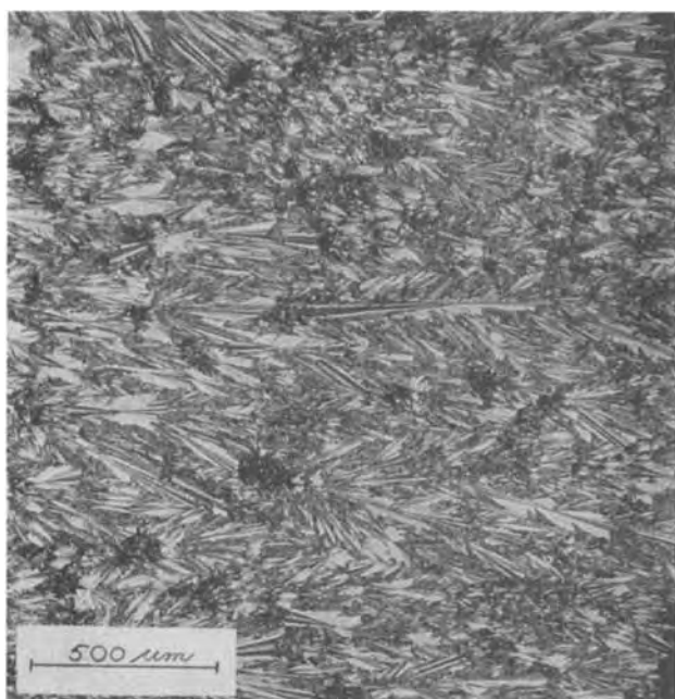
Fig. 2. Sample of silicon material B cut from a CVD grown bar. Growth direction is from left to right.
