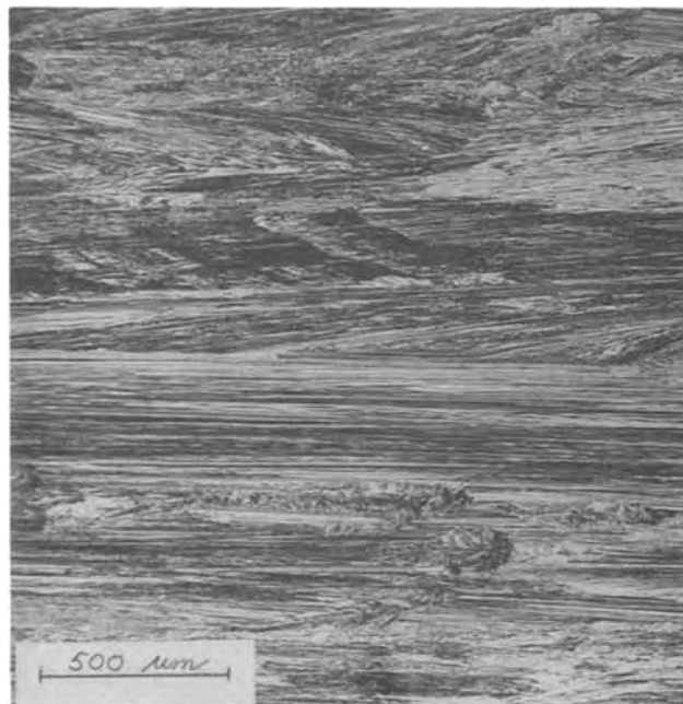
Fig. 1. Sample of silicon material A cut from a CVD grown bar. Growth direction is from left to right.
