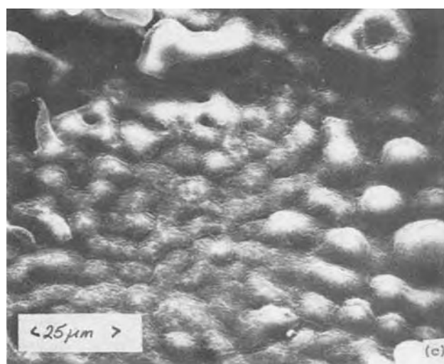
Fig. 3. Scanning electron photomicrographs of the elemental sulfur deposit on the stainless steel electrode after experiment 5 of Table I; (a) general surface, (b) upper layer deposit, (c) base layer deposit.
