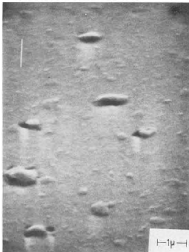
Fig. 2. Deposit observed on aluminum film exposed to a \text{CCl}_4 plasma using stainless steel electrodes. Plasma conditions were 67 Pa \text{CCl}_4 , 100W, 100^\circ\text{C} , and 2.5 cm electrode spacing.
