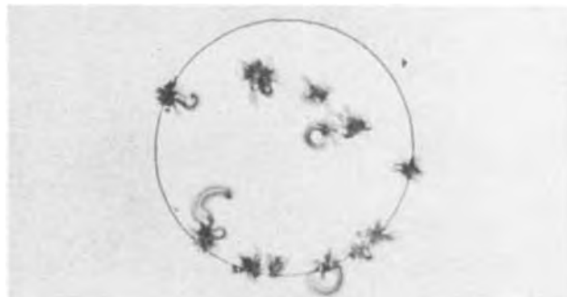
Fig. 5. After opening windows in the thick (steam) oxide, the thin (dry oxygen) oxide was grown. This thin oxide is contained within the circular area. It can be clearly seen that type II defects occur preferentially at the intersection of thin and thick oxides where a ledge in the silicon is situated (circle diameter = 168 \mu\text{m} ).
